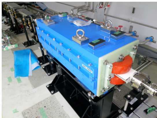
Kicker magnet (Yoke length 0.95 m, B_{\max}=0.9 T)
