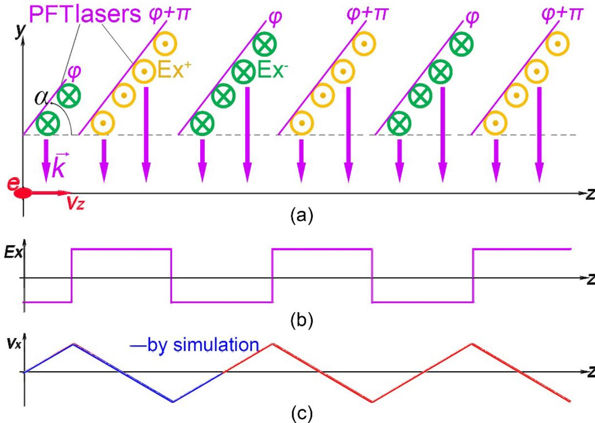
$$x(z) = -\frac{eE_x}{m_e\gamma} \frac{z^2}{2v_z^2} + \frac{v_0}{v_z} z + x_0$$
