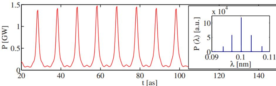
Thanks to mode locking, the FEL pulse has internal CEP stability.
