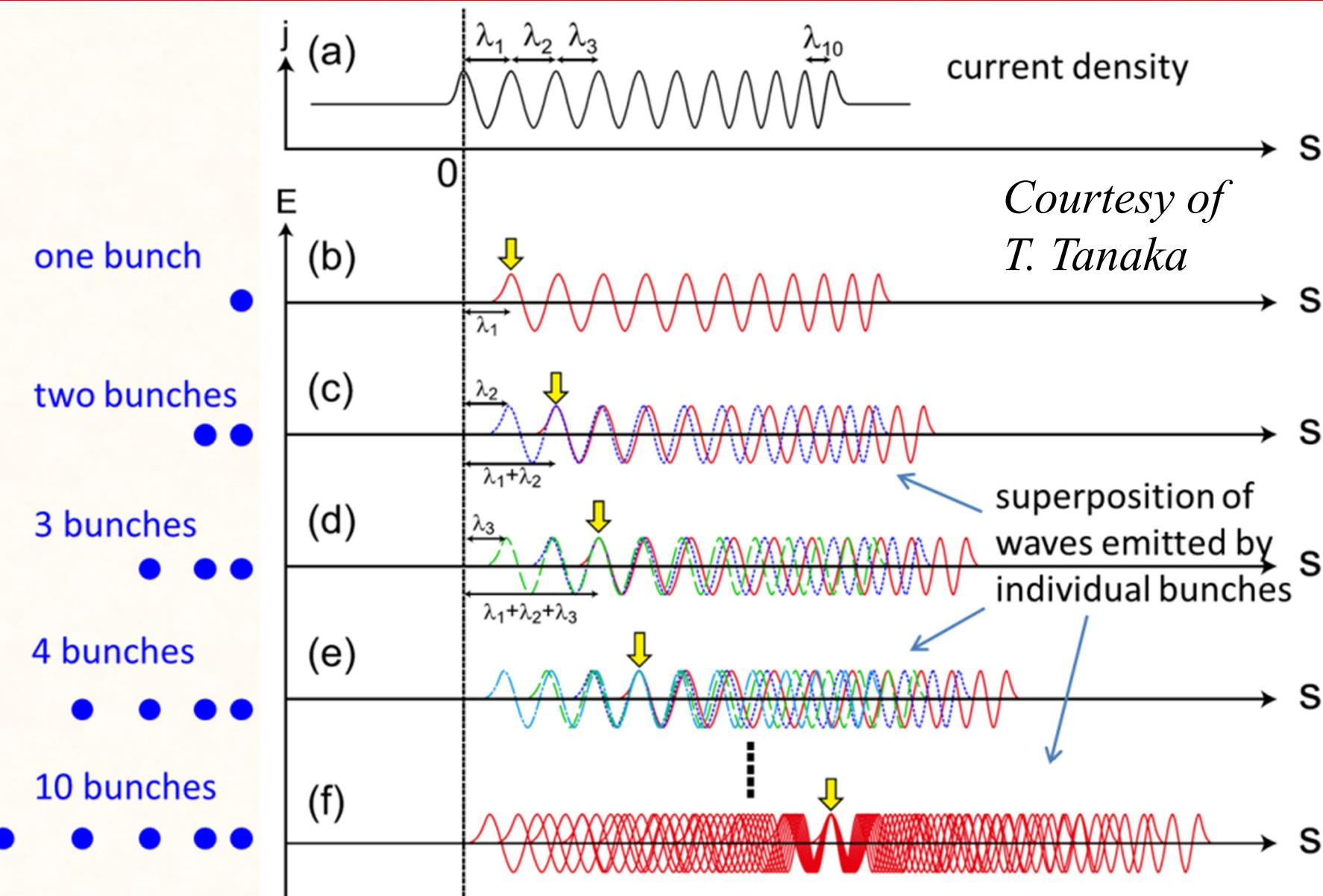
Pulse waveform can be controlled by taper profile.
