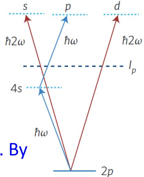
Two colors produce a beat wave with 105 as period. By adjusting the relative phase with 3 as precision, a quantum system is driven into a specific final state.
