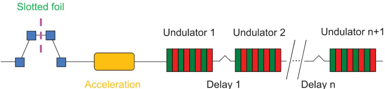
Uses a foil with multiple, unevenly located slots.
