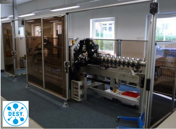
Cavity tuning machine (developed (w/ FNAL support) and handed over, and still maintained by DESY)
