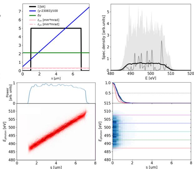
Figure 2: A 6  $\mu\text{m}$ -long flattop model electron beam with linear energy chirp, see top left plot, used to generate SASE radiation. It is dumped during the exponential growth for 500 statistically independent events. Subplots and notations identical to those on Figure 1.
