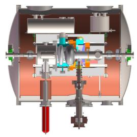
Figure 1: An overview of DC-SRF photocathode injector.
