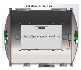
Figure 4: A layout of the magnetic shielding.
