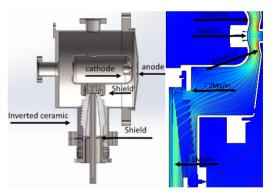
Figure 2: The new design of the DC structure (left) and electric field (right).
