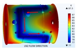
Figure 3: Temperature distribution of the 77 K copper screen.
