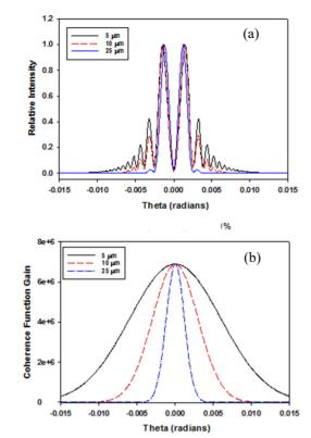
Figure 4: COTRI calculations for a) fringes and b) coherence function for beam sizes of 5, 10, and 25 µm.
