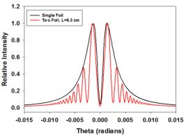
Figure 3: Comparison of far field OTR angular distribution patterns for a single foil and a two-foil interferometer. A beam energy of 375 MeV, wavelength of 266 nm, L=6.3 cm, and a divergence of  $\sigma_{\theta} = 0.1$  mrad were used in the calculations.
