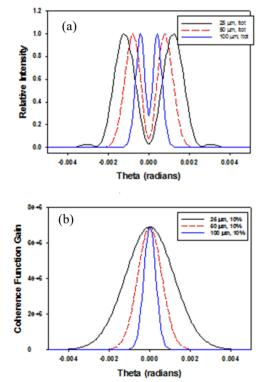
Figure 5: COTRI calculations for (a) fringes and (b) coherence function for beam sizes of 25, 50, and 100 µm.
