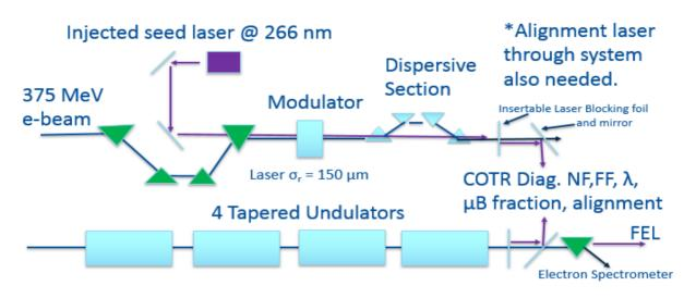
Figure 1: Schematic of the proposed LEA beamline layout showing the chicane, injected seed laser, modulator, COTR screens, undulators, and electron spectrometer.
