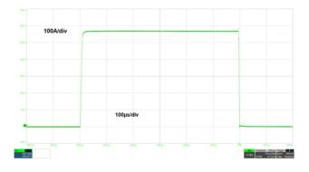
Figure 3: Example of current pulse.
