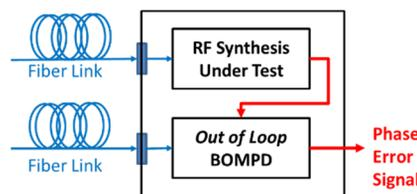
Figure 7: Measurement setup for relative timing jitter between the OMO and the RF synthesized signal using BOMPDP as out-of-loop phase detector.
