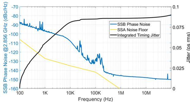
Figure 6: SSB phase noise for locked VCO, signal source analyzer (SSA) noise floor and absolute integrated timing jitter.
