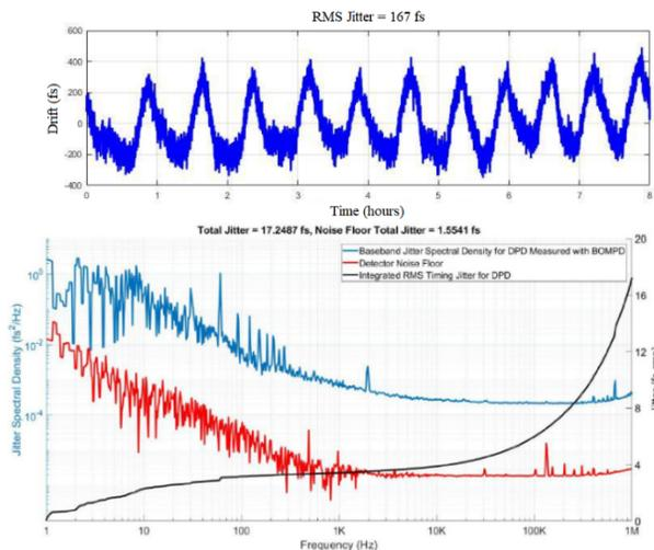
Figure 8: Timing stability of direct photodetected synthesis (a) Long term stability (b) Short term relative jitter given by Jitter Spectral Density.
