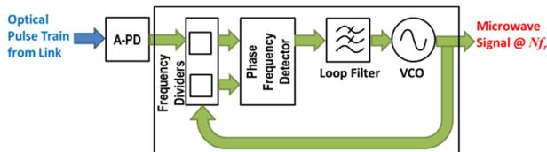
Figure 5: Digital VCO synchronization scheme for microwave synthesis.
