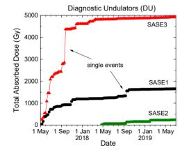
Figure 2: Total absorbed doses in the SASE1-3 Diagnostic Undulators up to July-2019.
