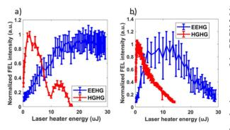
Figure 2: a) FEL energy vs laser heater energy at harmonic 18th. b) FEL energy vs laser heater energy at harmonic 2 30<sup>th</sup>.
