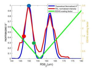
Figure 4: Normalized theoretical square bunching (blue), measured normalized FEL intensity (red) and ) EEHG scaling factor (green)vs R56 of the second dispersion section.
