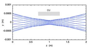
Figure 2: Symmetric beam trajectory satisfying a matched condition in the non-deflecting plane.
