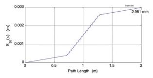
Figure 4:  $R_{56}$  variation along the beam line include the undulator. Straight lines at both sides are in drift spaces.
