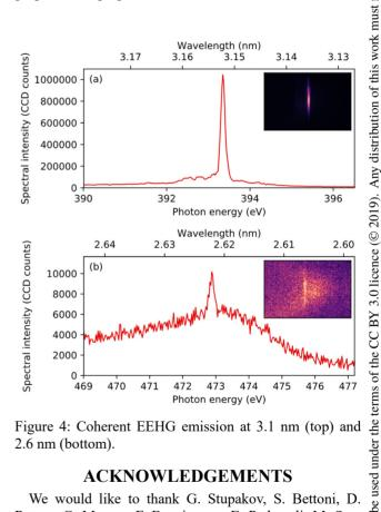
Figure 4: Coherent EEHG emission at 3.1 nm (top) and 2.6 nm (bottom).
