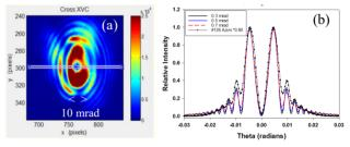
Figure 7: (a) Example of a FF COTRI image at 633±5 nm from the same shot as Fig. 5. (b) Comparison of the azimuthally averaged fringe data and the COTRI model for 0.3,0.5, and 0.7 mrad divergence. The fringe peak positions are well matched, but the relative intensities of some outer fringes are higher in the data. The best match is 0.5 mrad.
