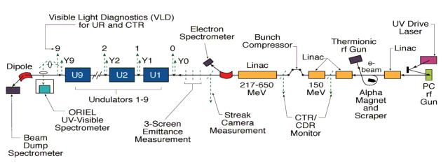
Figure 1: Schematic of the APS linac and SASE FEL beamline layout showing the UV drive laser, PC rf gun, linac, and SASE FEL undulators with diagnostic station locations circa 2002 [2].
