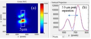
Figure 6: a) Vertically polarized NF image showing two pairs of coherent PSF lobes for two beamlets separated by about 6 µm. b) vertical profile of right hand beamlet with a 5-µm lobe separation which is mapped to 4.6 µm (FWHM) or 2.0 µm (σ).
