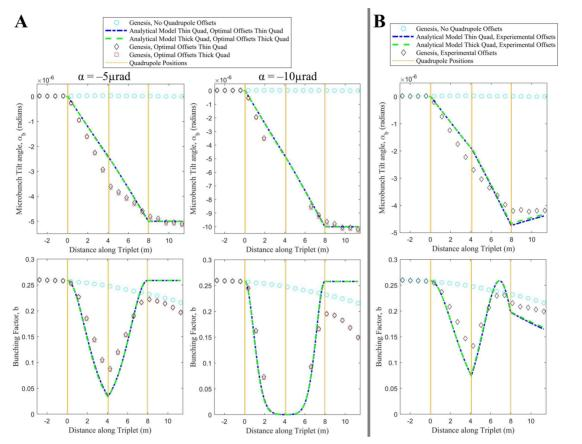
Figure 2: Microbunch tilt angle in nonrotated frame,  $\alpha_b$  and bunching factor, b, through an quadrupole triplet. are A) analytical model optimal using thin or thick quadrupoles, or B) replicating a 2018 experiment.
