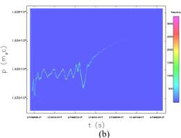
Figure 5: Longitudinal phase space of the beam at the linac exit, with laser heater on (a) and off (b)
