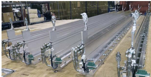
Figure 6: Five HXR chambers assembled in alignment fixtures with water fittings and Earth-field coils.
