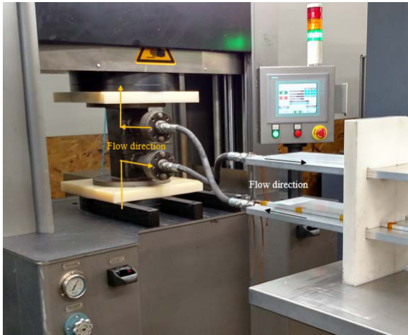
Figure 2: The right angle diverter showing flow direction.
