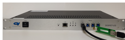
Figure 1: DOSFET-L02 controller and sensor mount module from Elettra-Sincrotron Trieste.
