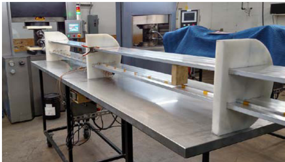
Figure 4: Photo of the setup. Behind this setup is a second identical setup under an insulating blanket during processing. Also shown here are the roller brackets that also hold the heaters in place.
