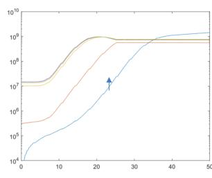
Figure 8: Semi-log plots of SASE (blue), pass 2 (orange), pass 3 (yellow), pass 4 (green) and pass 5 (purple). The SASE simulation is stopped at the 7<sup>th</sup> undulator (arrow).
