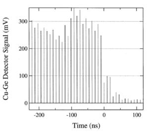
Figure 3: Ring-down of the IR RAFEL energy. The pulse energy decreases to one-third its initial value in one pass.
