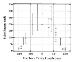
Figure 4: Cavity detuning length of the IR RAFEL.
