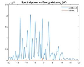
Figure 9: SASE and filtered signal on a linear scale. The Gaussian-shaped filter selects only 6% of the spectral power within a single SASE spike as the coherent seed for amplification in Pass 2.
