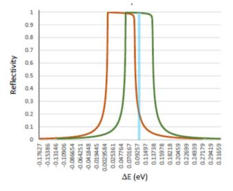
Figure 6: Reflectivity versus energy detuning from Bragg for diamond (400) at 20°C (green) and 45° (orange).
