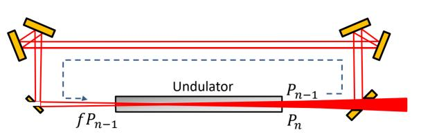
Figure 1: Schematic of the IR RAFEL. The optical feedback cavity consists of six copper mirrors, two flat annular mirrors and two pairs of curved mirrors. The electron beam travels from the left through the two annular mirrors and the undulator.
