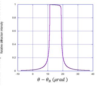
Figure 5: Calculated rocking curve for diamond (400).
