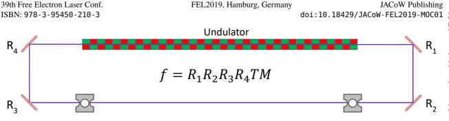
Figure 7: Schematic of an X-ray RAFEL. The feedback fraction f is the product of the four mirror reflectivity (R<sub>1</sub> through R<sub>4</sub>), the combined transmission T of the two compound refractive lenses (CRL) and the spectral power fraction selected by the Bragg mirrors M within the cavity angular acceptance as defined by the radiation mode over the CRL separation.
