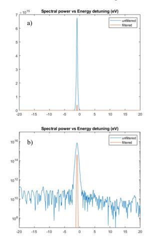
of Figure 10: Plots of spectral power in Pass 5 versus energy under the terms detuning in eV on linear (a) and log (b) scale.
