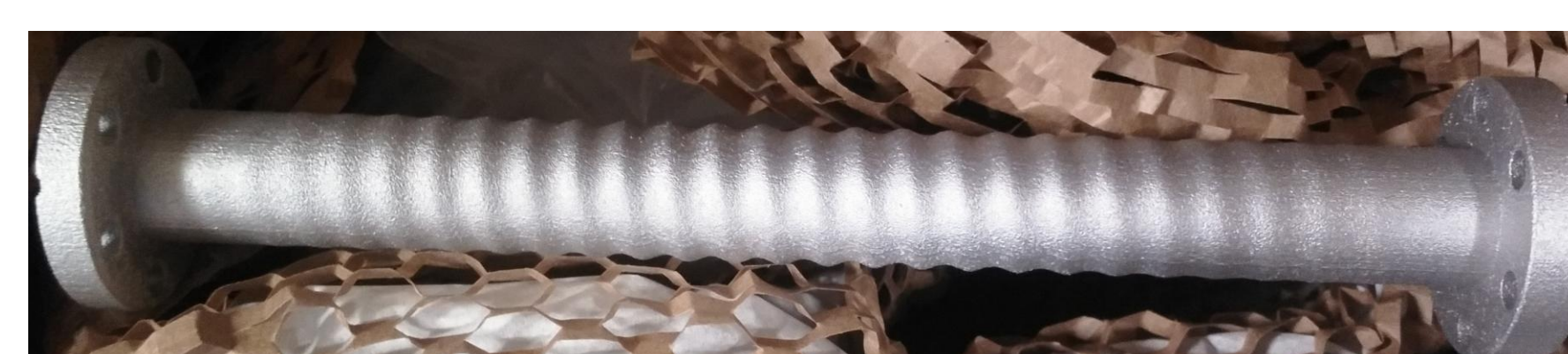
A 34 GHz TE 11 -TM 01 -TM 11 RF undulator.
