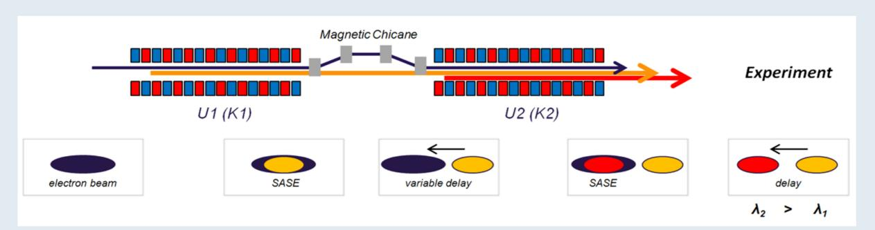
Inserting an optical delay allows for scanning through zero delay
