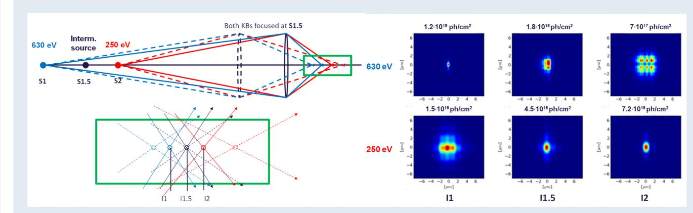
Reimaging artificial intermediate source S1.5 onto the sample, assumed at I1.5 allows to minimize aberrations and obtain comparable radiation size and photon flux density (reaching beyond 10<sup>18</sup> photons/cm<sup>2</sup> per pulse).
