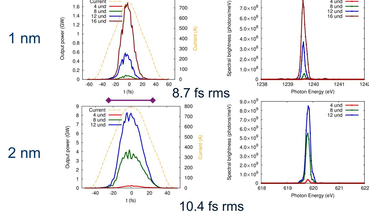
at 2 nm, pulse can be as short as 7.5 fs rms with a 25 fs bunch
