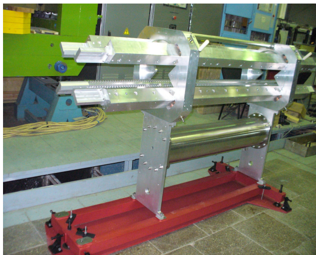
Figure 5: Assembled undulator. The extensions at the ends of the cassettes are installed for magnetic measurements.
