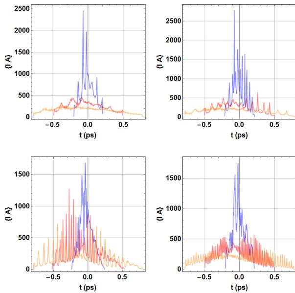
Figure 4: Current profiles for scans of bunch compression factor for the laser intensity profiles given in Fig. 3: Blue: 1.4; Red: 3.0; Orange: 4.6.
