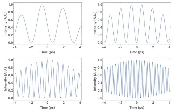
Figure 3: Calculated intensity profiles of modulated laser pulses for: Top left: 1 ps; top right: 2ps delay; bottom left: 4ps delay; bottom right: 8ps delay.
