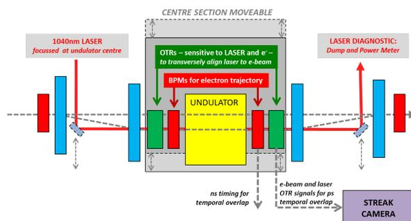
Figure 1: Schematic of laser heater system. Dipoles are shown in blue.
