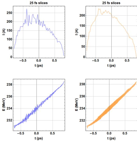
Figure 2: Current profiles at full energy for: Left: laser heater off; Right: laser heater at nominal settings.
