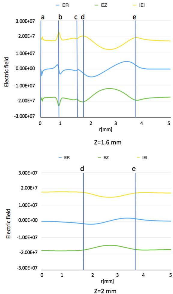
Figure 6: Electric field on the r-axis for different planes in the z-axis:  $z = 1.6$  mm (upper plot) and  $z = 2$  mm (lower plot). Individual points represent roughness on the surface: a) 50- $\mu\text{m}$  bump, b) 30- $\mu\text{m}$  bump, c) 30- $\mu\text{m}$  bump, d) and e) the photocathode RF gun arc.
