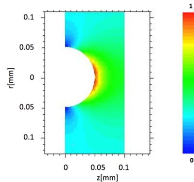
Figure 5: Normalized contour of electric field amplitude in POLFEL gun on the 50  $\mu\text{m}$  bump.
