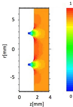
Figure 3: Magnitude of the electric field in the vicinity of the cathode plug.
