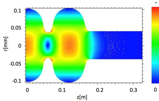
Figure 2: Simulated magnitude of the electric field in the e-gun cavities.
