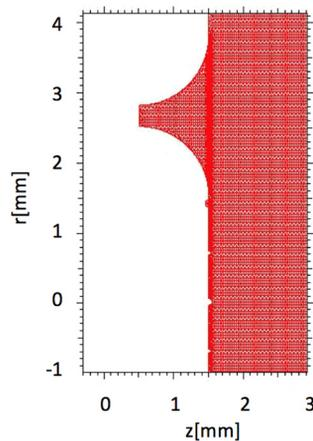
Figure 4: Mesh of photocathode in FEM program.
