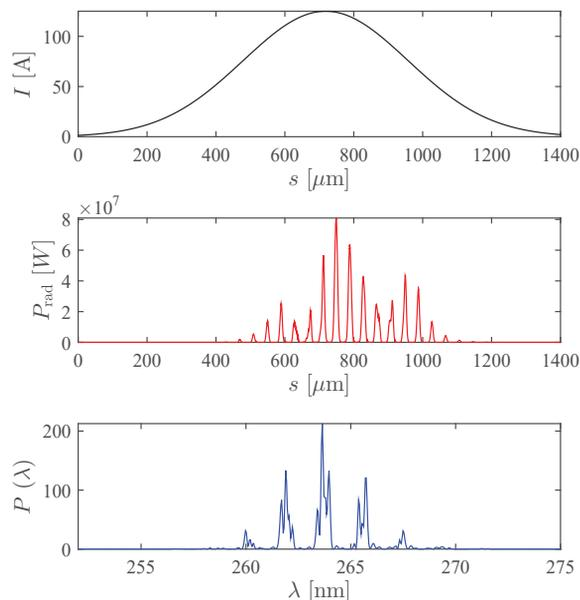
Figure 2: Current profile (top), temporal profile of the FEL power after 15 undulator modules (middle) and corresponding spectrum (bottom).
