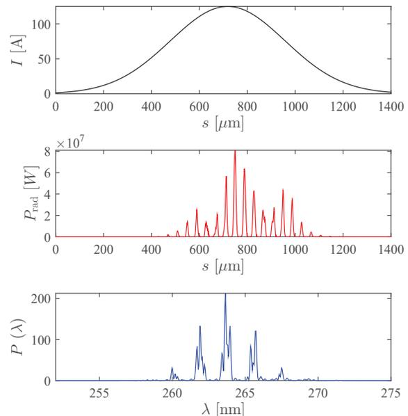
Figure 2: Current profile (top), temporal profile of the FEL power after 15 undulator modules (middle) and corresponding spectrum (bottom).
