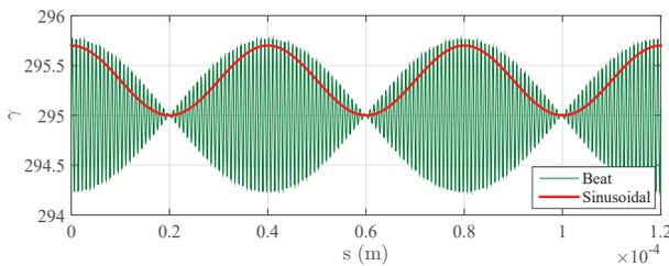
Figure 1: Electron beam energy variation with longitudinal bunch position for a beat modulation case comprising two sinusoidal wavelengths of  $\lambda_1 = 800$  nm and  $\lambda_2 = 816$  nm to give  $\lambda_{\text{beat}} = 40$   $\mu\text{m}$  and a sinusoidal modulation with  $\lambda_{\text{mod}} = 40$   $\mu\text{m}$  as typically used in mode-locked FEL simulations.
