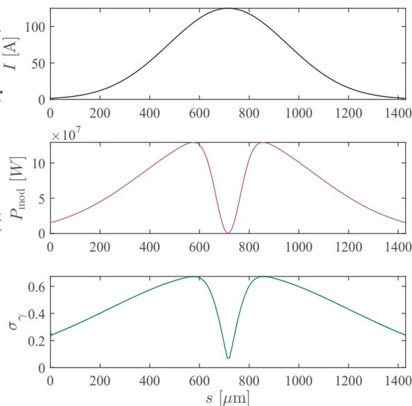
Figure 3: Current profile (top), temporal profile of the modulating laser pulse (middle) and corresponding induced energy spread at the end of the modulator (bottom).
