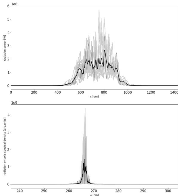
Figure 5: Nominal case power (top) and spectrum (bottom) for 10 shot noise cases (grey) and the average (black).
