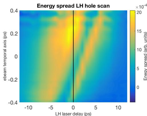
Figure 3: False colour plot representing the slice energy spread produced by the LH laser as a function of the laser delay with respect to the electron beam.
