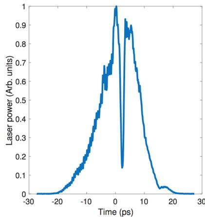
Figure 2: Cross correlation curve of the LH laser pulse with the temporal shaping. A narrow region in the centre of the pulse is characterized by low intensity.
