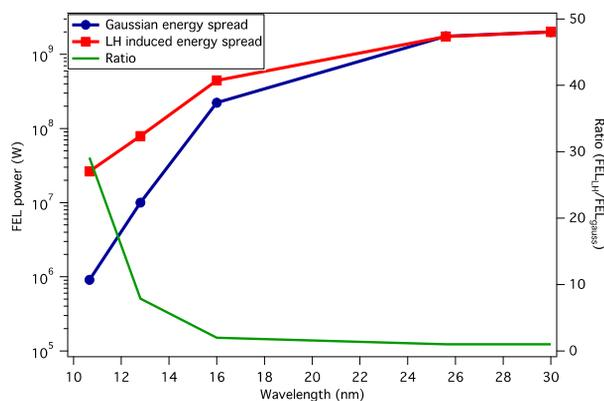
Figure 1: Simulations results of FEL power vs wavelength for standard Gaussian energy spread and LH induced non-Gaussian energy spread [16].
