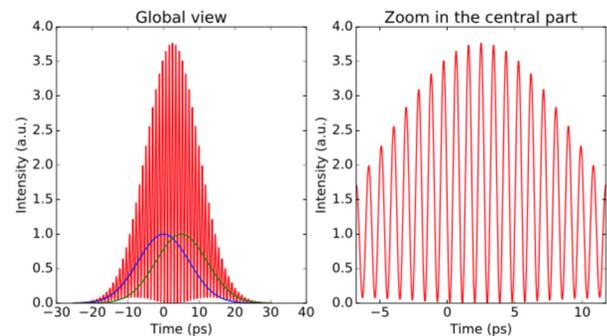
Figure 4: Amplitude modulated laser pulse obtained with the beating from two chirped pulses with a small relative delay.
