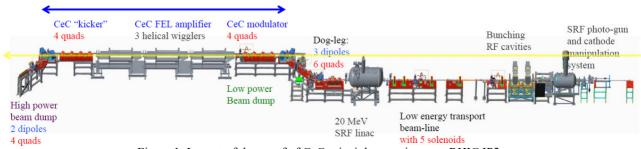
Figure 1: Layout of the proof of CeC principle experiment at RHIC IP2.
