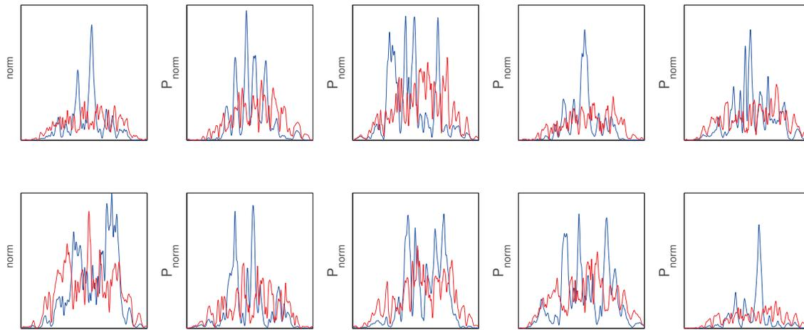
Figure 5: SHORT mode stabilisation: 10 randomly chosen examples from the 24 different shot noise seeds, showing the SASE (blue) and stabilised (red) pulse profiles at the exit of the 8th undulator module. Each pulse is normalised such that the pulse energy is unity.
