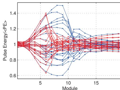
Figure 4: SHORT mode stabilisation. The blue plots show the 24 individual SASE cases, where the pulse energy at each module is normalised to the mean SASE pulse energy at that module. The red plots are for the 24 stabilised SASE cases.
