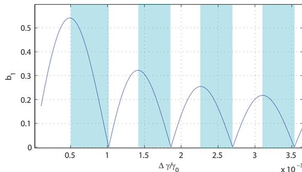
Figure 1: Plot  $b_n$  vs  $\Delta\gamma/\gamma_0$  using Equation (1), for  $\sigma_b = 1 \times 10^{-4}$ ,  $\lambda_r = 2\pi/k_r = 100$  nm,  $n = 1$ , and  $R_{56} = 60$   $\mu\text{m}$ . The blue shading highlights regions where the gradient of the function is negative.
