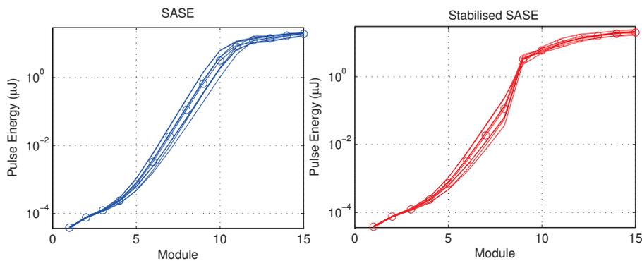
Figure 2: ULTRASHORT mode stabilisation. Top left shows the pulse energy growth for a control SASE case, with 8 different shot noise seeds. The circles mark the average. Top right shows the results where chicanes are applied before undulator modules 9, 10 and 11, with  $R_{56}$  values empirically optimised to 60  $\mu\text{m}$ , 20  $\mu\text{m}$  and 5  $\mu\text{m}$ .
