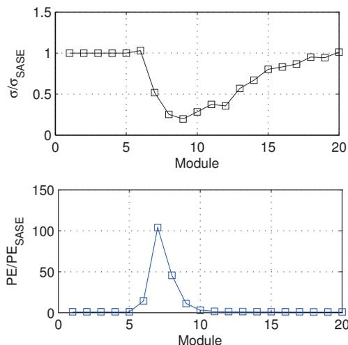
Figure 3: SHORT mode stabilisation. Top shows the RMS variation of the pulse energy over the 24 different seeds for the stabilised case, normalised to the SASE control case, and bottom right shows the normalised average pulse energy growth
