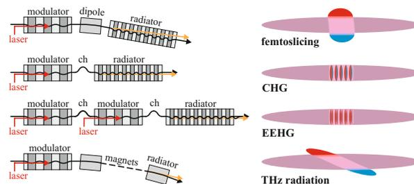
Figure 1: Applications of laser-induced energy modulation in storage rings. Left: Magnetic layout with undulators and chicanes (ch). Right: Resulting electron bunch structure (red and blue: electrons with energy gain and loss).
