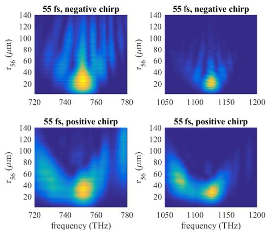
Figure 3: CHG spectra of the second (left) and third harmonic (right) of 800 nm seed pulses with negative chirp (top) and positive chirp (bottom), both with a pulse length of 55 fs, under variation of the chicane strength  $r_{56}$ .
