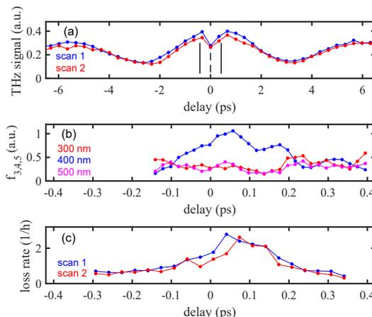
Figure 5: THz radiation (a), Fourier coefficients of the THz signal for few-fs delay variation (b), and beam loss rate (c) as function of the delay between 800 and 400 nm seed pulses. Zero delay and the delay range of (b,c) is defined in (a).
