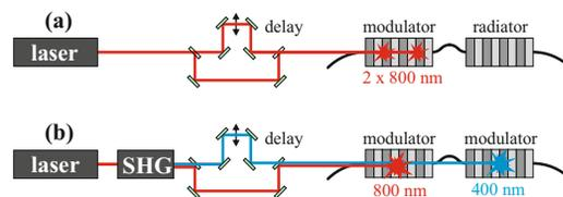
Figure 4: Seeding with 800 nm double pulses in the same modulator (a) and with 800 and 400 nm pulses in two modulators (b) with variable delay.
