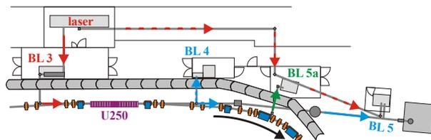
Figure 2: The short-pulse facility at DELTA comprising a laser system, a laser beamline (BL 3) guiding seed pulses to the undulator U250, a diagnostics beamline (BL 4), a soft-X-ray beamline (BL 5), and a THz beamline (BL 5a).
