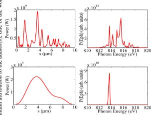
Figure 1: The FEL power at  $U_1$  and monochromatic stage in time (top) and frequency (bottom) domain. At the exit of U<sub>s</sub> (left); At the exit of monochromator (right).
