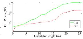
Figure 2: The fundamental (green line) and  $3^{rd}$  (red line) harmonic power evolution along the radiator undulator  $U_2$
