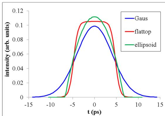
Figure 2: Used pulse profiles for the three types of photocathode pulse envelopes.
