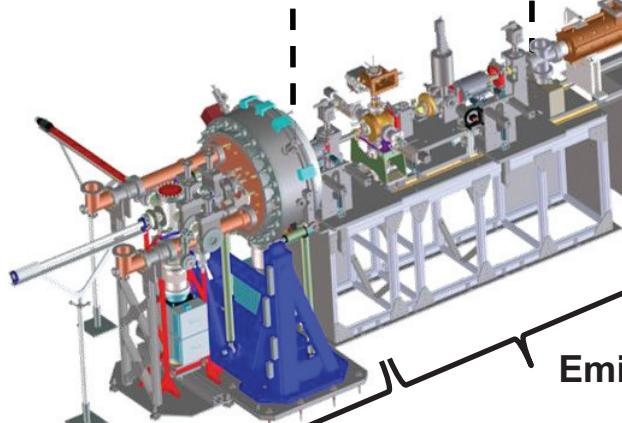
1.3 GHz copper accelerating cavities (pulsed), diagnostics systems
