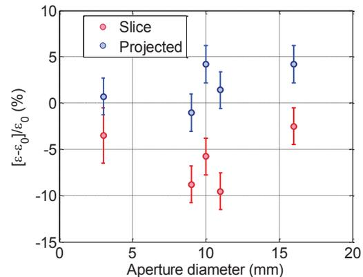
Figure 12: Projected emittance with respect to the case without the collimator as a function of the hole diameter. The central slice emittance is reported for comparison.
