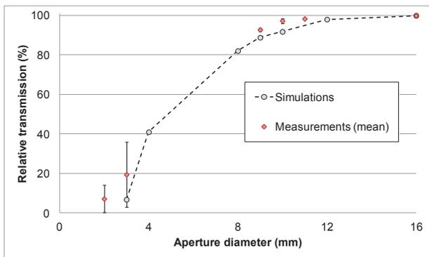
Figure 10: Charge transported at the end of SITF with the CTF2 gun as a function of the collimator aperture hole compared with the simulations. The charge is normalized to the transmitted charge without the collimator. The error bars are calculated from the difference of several sets of measurements.
