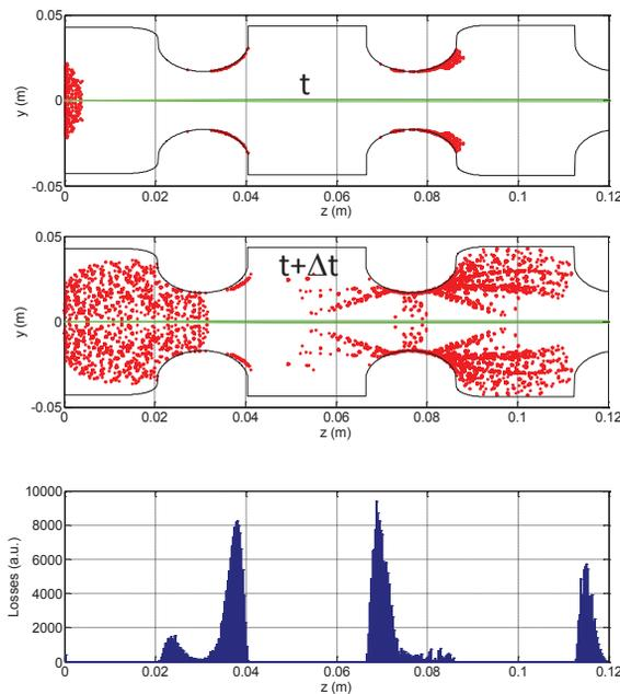
Figure 2: Simulated dark current in the SwissFEL gun during the emission. The locations of the losses in the gun are also indicated.
