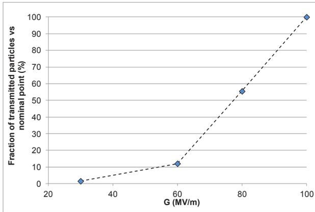
Figure 5: Dark current transmission as a function of the gun peak field on the cathode.
