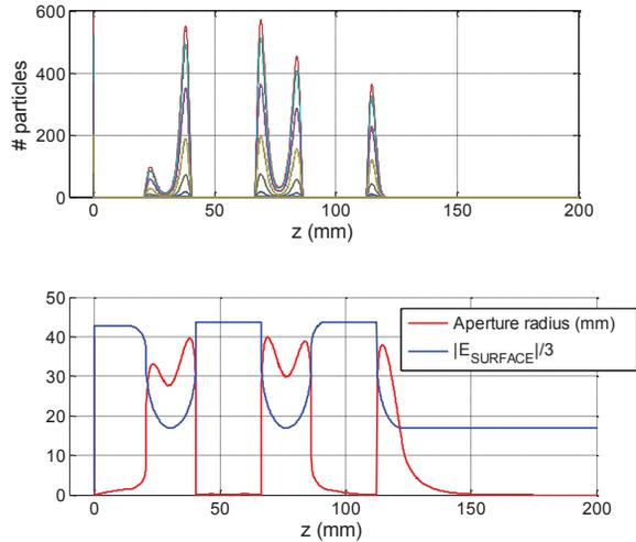
Figure 1: Macroparticles emitted according to the emission model. Each colour corresponds to a 9 degrees time step in one RF period (upper plot). Gun geometry and surface electric field on the aperture (bottom plot).
