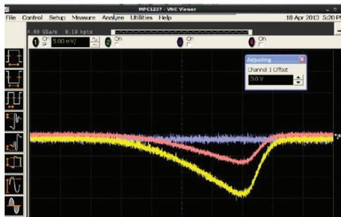
Figure 6: Signals from the Faraday cup during the measurement. Yellow trace: raw signal. Blue trace: background. Pink trace: signal after background subtraction. H-step = 200 ns/division.
