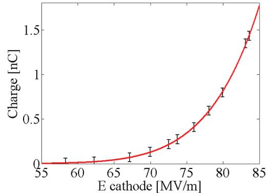
Figure 7: SITF gun charge emission as a function of peak cathode field. Solid line: fitting, black point: experimental data.
