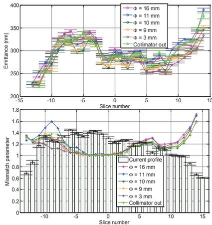
Figure 13: Emittance along the bunch, mismatch parameter and current profile for the several diameter holes.
