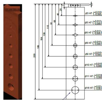
Figure 8: Collimator plate installed in SITF.
