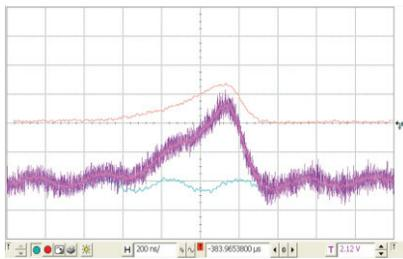
Figure 9: Oscilloscope reading of the 10 mm aperture measurements. Pink trace: raw signal. Cyan trace: background. Light pink: signal after background subtraction. H-step = 200 ns/division.
