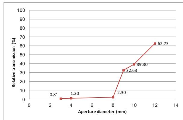
Figure 4: Transmission of the dark current renormalized to the transmission without the collimator.
