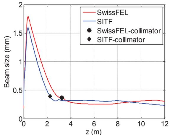
Figure 3: rms beam size of the 200 pC nominal beam and position of the collimators in the SITF and in the SwissFEL case.
