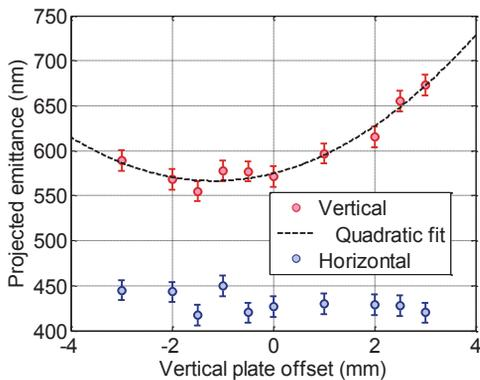
Figure 14: Vertical and horizontal projected emittance as a function of the plate vertical offset. A second order dependence of the emittance with respect to the beam offset is expected by the theory.
