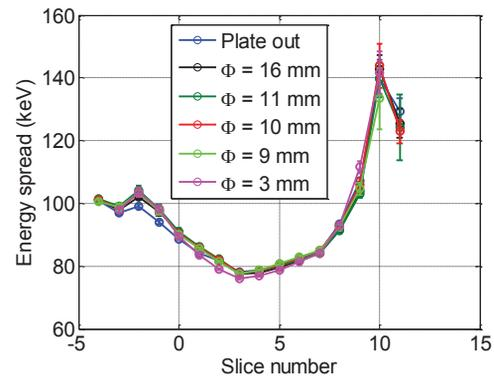
Figure 11: Slice energy spread measured for several collimator apertures along the bunch.
