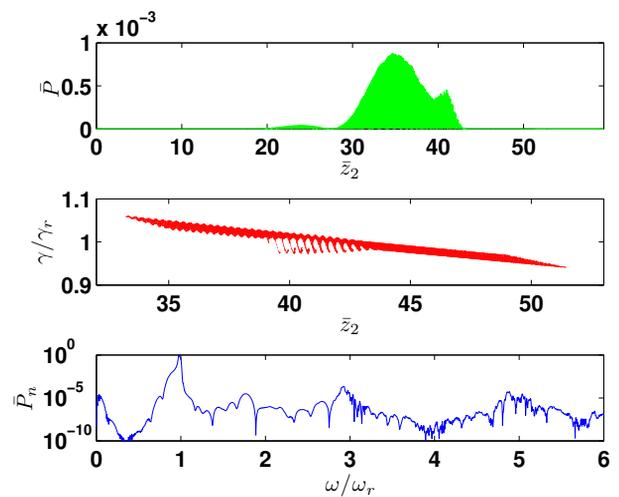
Figure 1: Scaled Power (top), electron phase space (middle) and scaled spectral power (bottom) from a 1D simulation of the parameters in Table 1. (Note the different scale in  $\bar{z}_2$  for the plot of electron phase-space).
