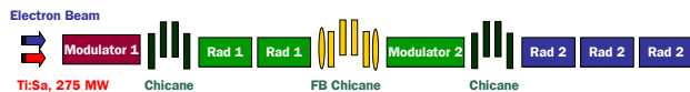
Figure 5: Schematic of the STARS HGHG cascade (note that the quadrupoles between undulators are not shown.)
