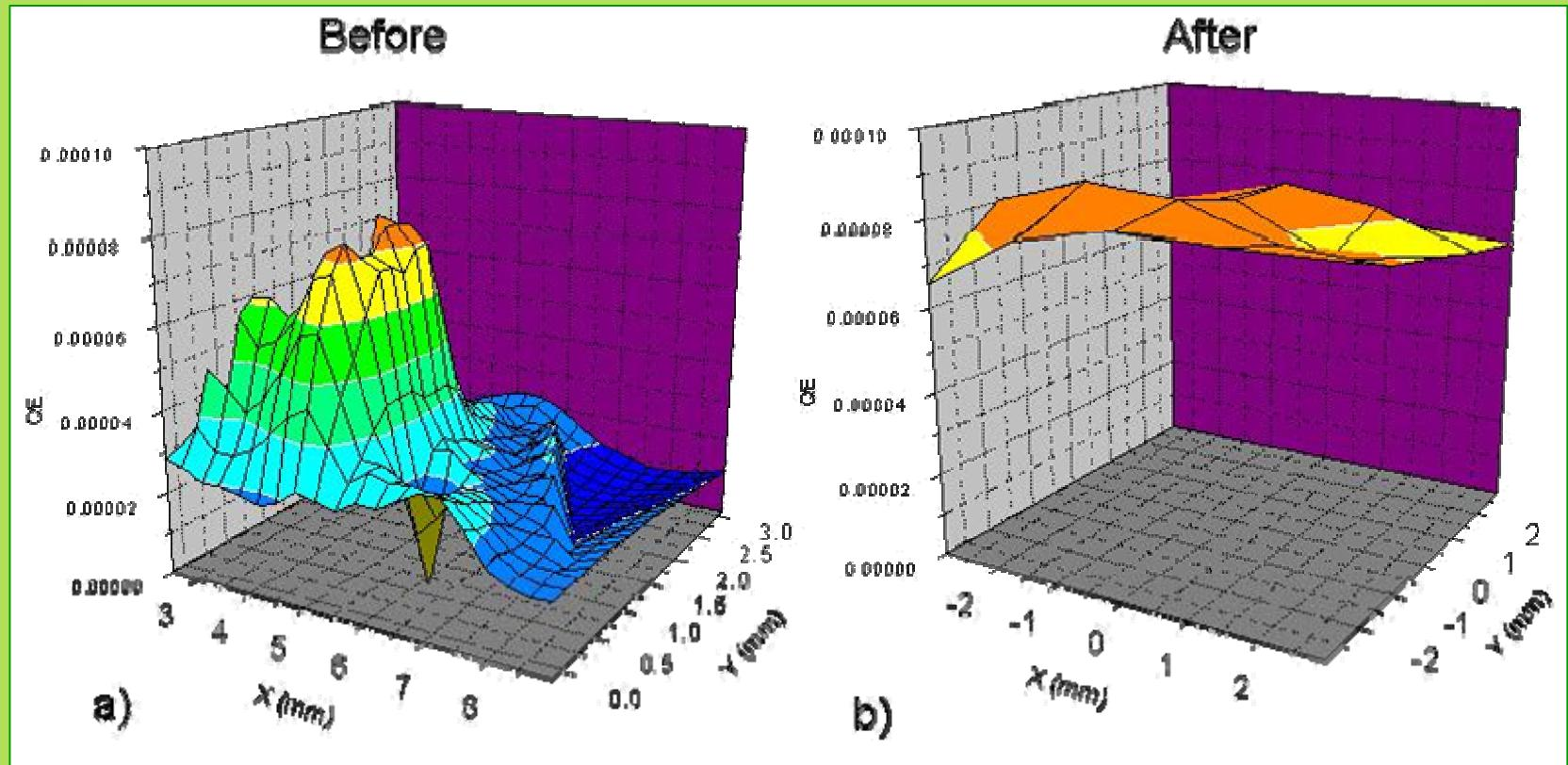
Laser cleaning with  $10 \mu\text{J}$  and  $100 \mu\text{m}$  spot size diameter.
