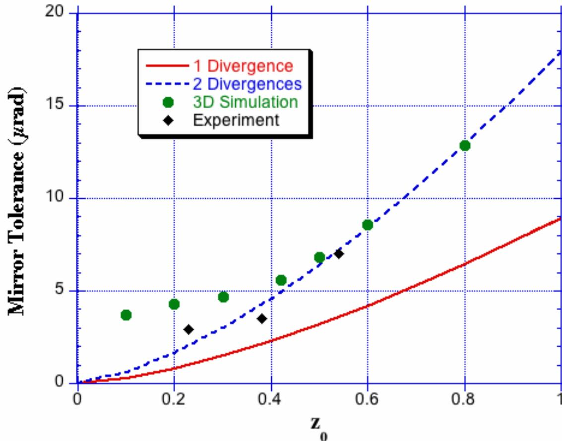
HWHM of the gain vs. mirror steering. The red curve is proportional to the crude mode-rotation model.
