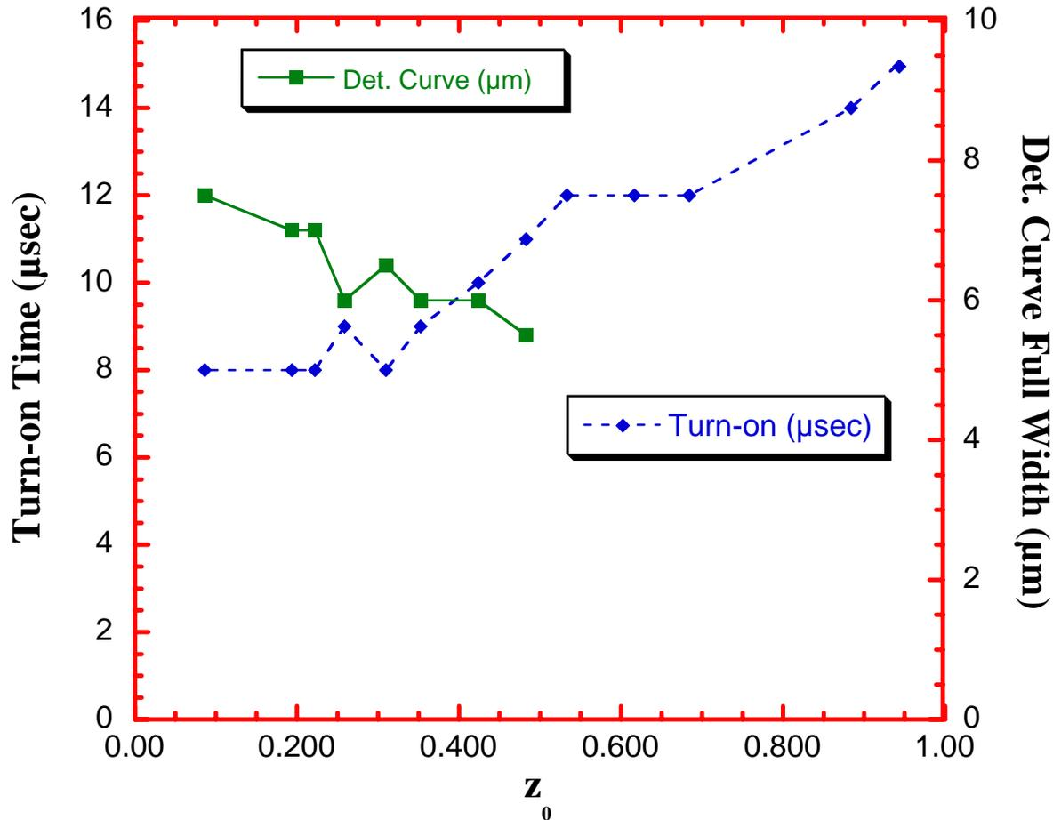
Detuning curve width should be proportional to gain. Turn-on time should be inversely proportional to gain.
