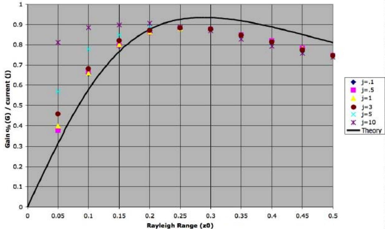
Figure 24. Gain curves for various Rayleigh lengths and dimensionless current values
