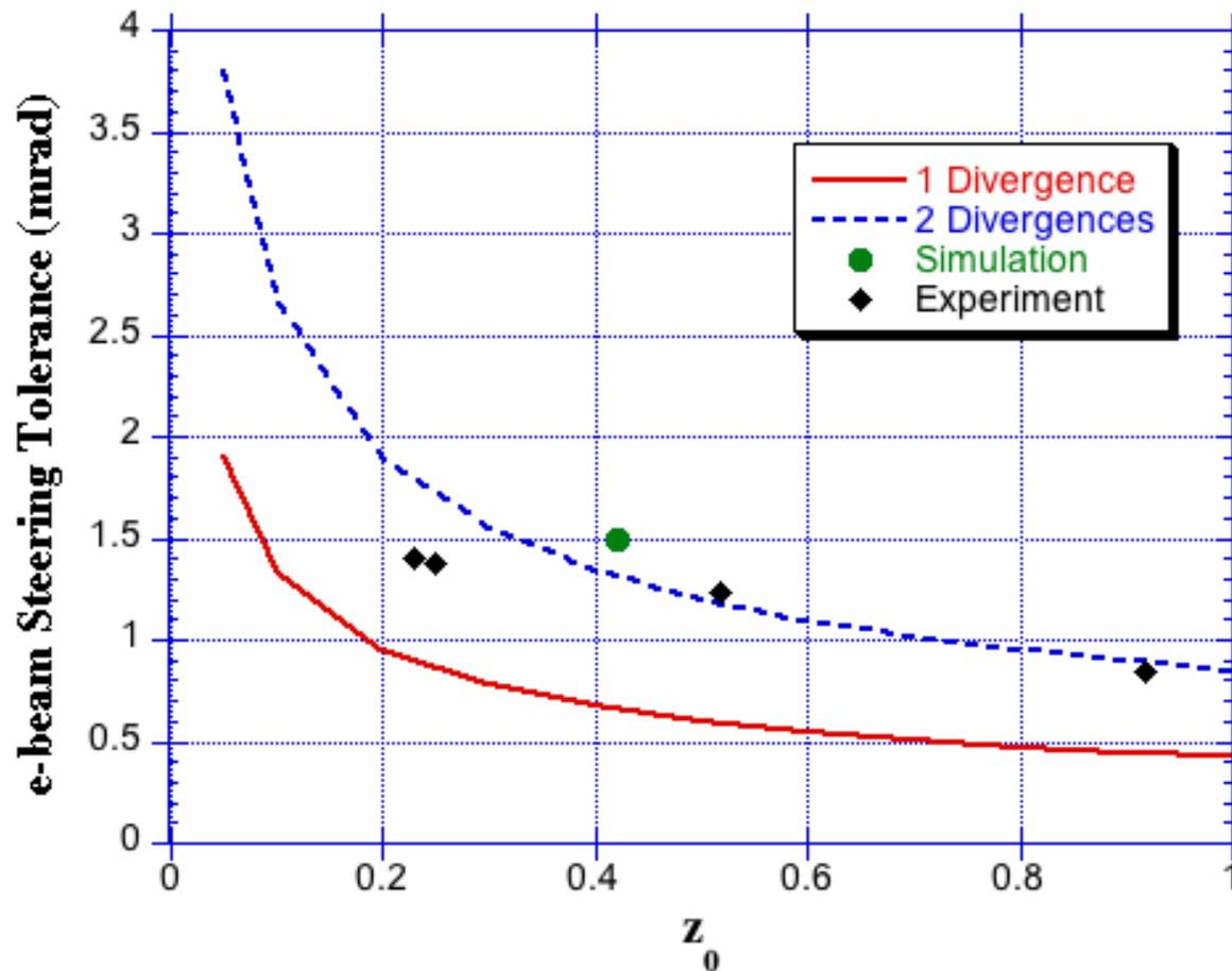
HWHM of gain vs. electron beam steering. The red curve corresponds to the crude mode-rotation model.
