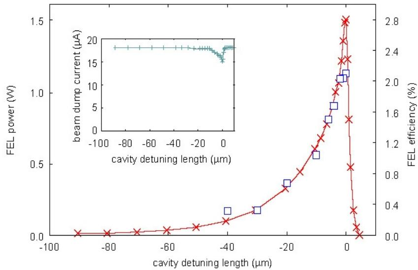
Figure 3: FEL power measured as a function of  $\delta L$  at macropulse length of  $230 \mu\text{s}$ . FEL efficiencies obtained from the energy distributions of the exhausted electron beam are shown by open squares. The efficiencies near zero detuning length cannot be measured with our energy analyzer due to the limited energy acceptance, and they are determined from measured FEL power. The inset shows the beam dump current with respect to  $\delta L$ .
