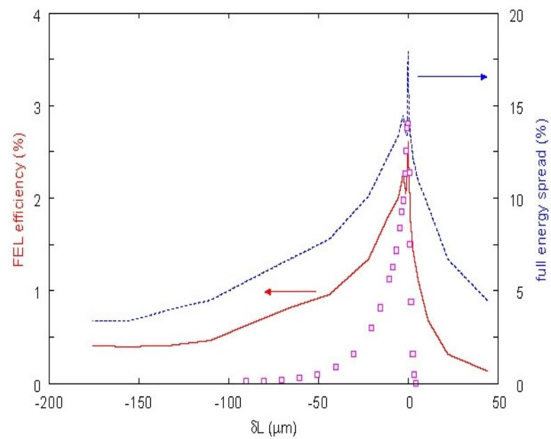
Figure 4: FEL efficiencies as a function of  $\delta L$  obtained from a one-dimensional time-dependent FEL simulation (solid line) and corresponding beam energy spread (dotted line). Measured FEL efficiencies are also plotted as open squares for comparison.
