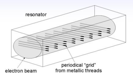
Theoretical analysis\* showed that periodic metal grid does not absorb electromagnetic radiation and the "grid" photonic crystal, made of metal threads, is almost transparent for the electromagnetic waves in the frequency range from GHz to THz.
