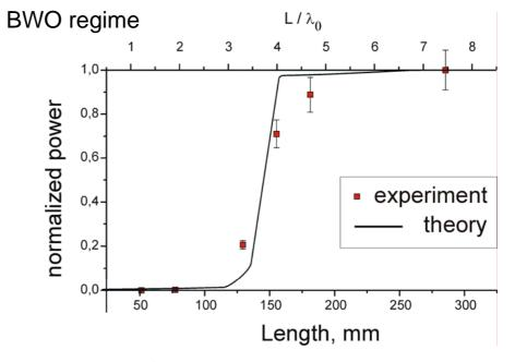
Dependence of radiation power on resonator length
