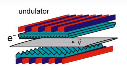
VFEL can use any spontaneous radiation mechanism (magnetic bremsstrahlung in undulator, radiation in laser wave, Smith-Purcell, diffraction or Cherenkov radiation and so on).
