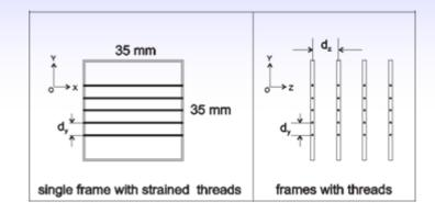
The "grid" structure is made of separate frames each containing the layer of 5 parallel threads with the distance between the next threads  $d_y$ =6 mm), 12 frames were joined to get the "grid" photonic crystal with the period 12.5 mm and another 12 frames formed "grid" photonic crystal with the period 10.5 mm .
