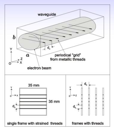
The "grid" structure is made of separate frames each containing the layer of 1, 3 or 5 parallel threads with the distance between the next threads  $d_y$ =6 mm). Frames are joined to get the "grid" structure.
