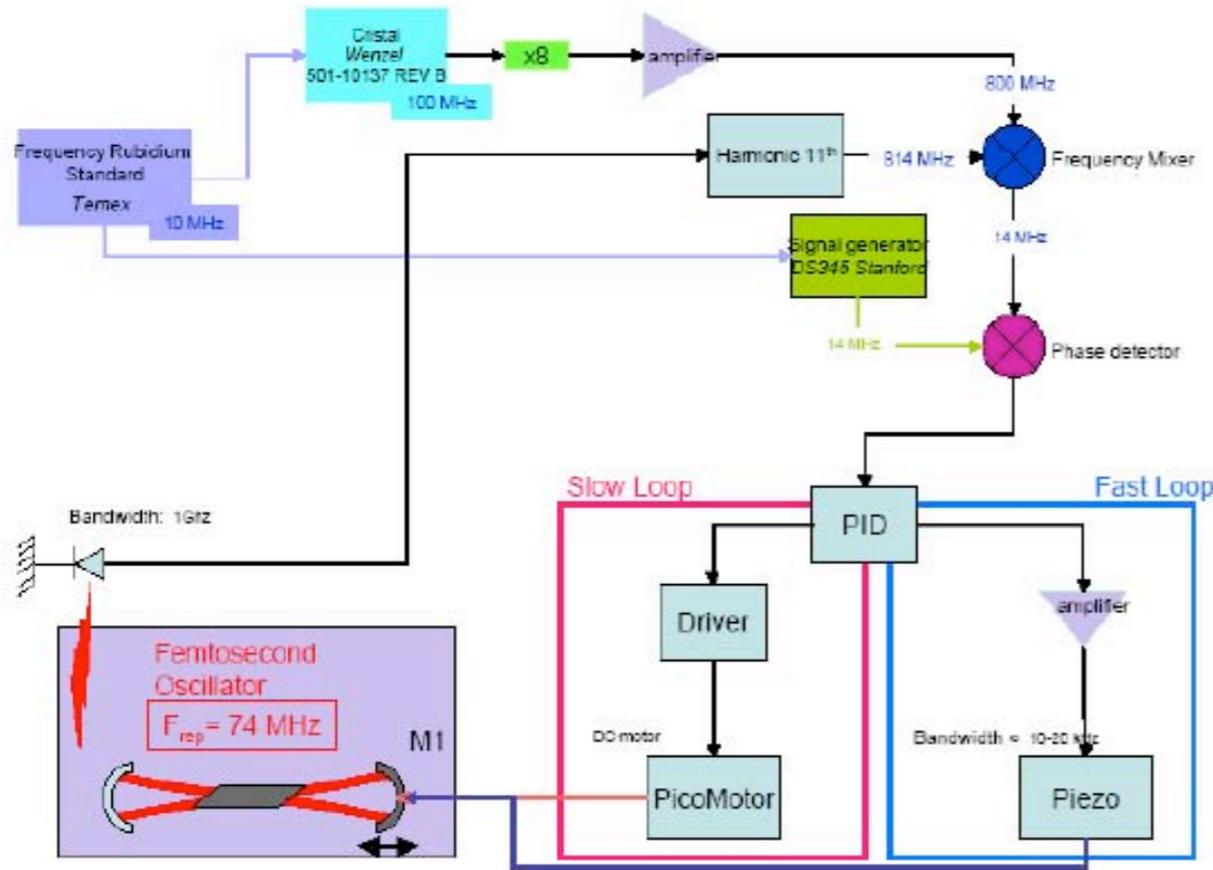
System of frequency stabilisation of the Ti:Sa oscillator with a reference given from an atomic clock
