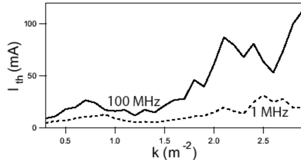
Threshold versus the strength of the quadrupoles
