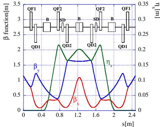
Figure 5: the optics design of bunch compressor
