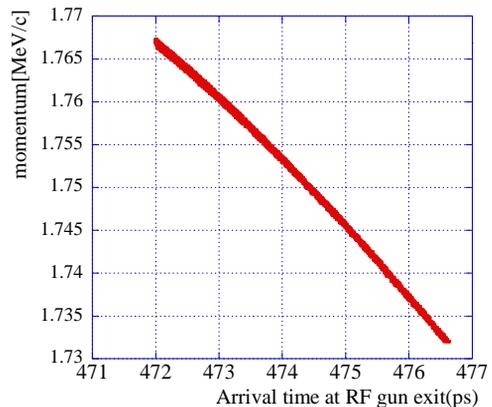
Figure 4: Longitudinal phase space distribution (FDTD simulation)
