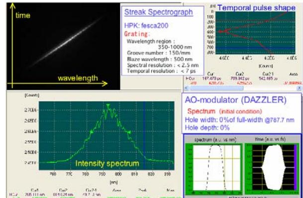
Figure 5: Initial intensity spectrum and chirp of the fundamental of Ti: Sapphire laser (after the stretcher): The linear chirp is measured by monochromator combined with streak camera (Hamamatsu Photonics K.K.)
