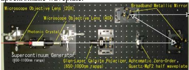
Figure 4: Supercontinuum generator (650-1100 nm) and broadband transport optics
