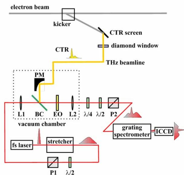
Figure 1: Set-up for electro-optic spectral decoding measurements of coherent transition radiation (CTR). Notations: ( $1/2$ ), ( $1/4$ ) – half and quarter wave plates; (P1,2) – polarizers; (L1,2) – lenses; (BC) – indium tin oxide beam combiner; (EO) – 0.5 mm thick ZnTe electro-optic crystal; (PM) – parabolic mirror
