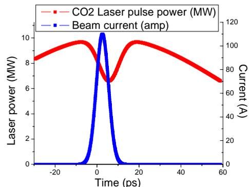
Figure 5: Beam loading in the 7th harmonic IFEL accelerator for a 100 Amp beam current and 12.3 MeV input energy. The beam current longitudinal profile is also shown.
