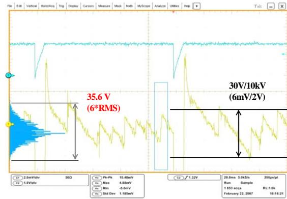
Figure 4: Regulating waveform of PFN voltage at the level of 10 kV with a PFN capacitance of 1.4  $\mu$ F. The accumulation time for statistical distribution of PFN voltage is 1 hour.
