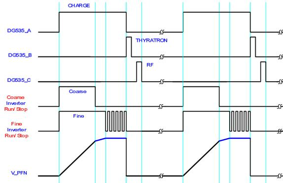
Figure 3: Timing diagram of the modulator control.
