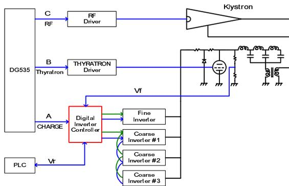
Figure 2: Schematic diagram of the modulator control.
