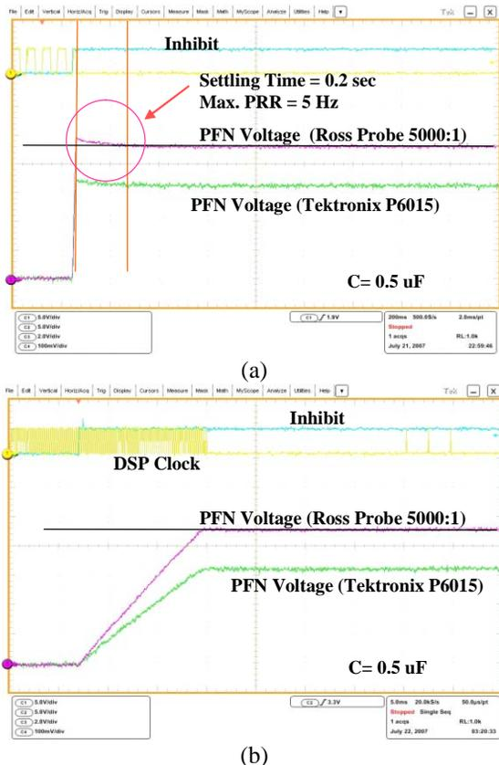
Figure 7: Digital control of charging overshoot. (a) The charging is done with a digital filter. (b) The charging is done with digital control of a charging pulse rate.
