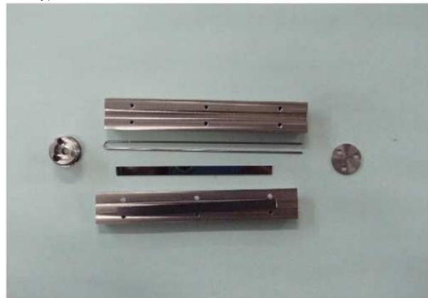
Figure 8: The double-slab resonator
