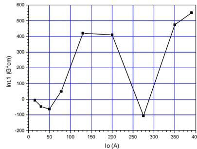
Figure 5: Final first field integral as function of the main coil excitation current
