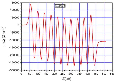
Figure 8: Magnetic field second integral for  $I_0=435$  A
