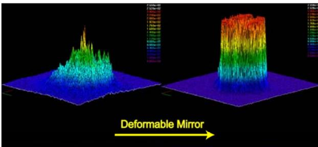
Figure 6: Result of spatial profile optimized to Top-hat with a deformable mirror (Laser profile monitor: LBA300-PC). The figures are normalised with the peak intensity to avoid saturation of laser profiler pixels.
