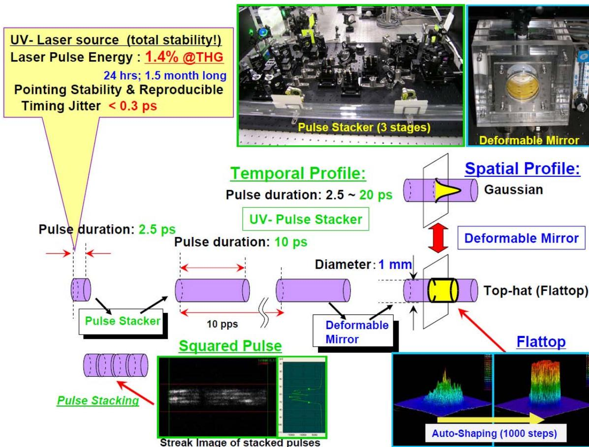
Figure 3: Three-dimensional (spatially (2D) and temporally (1D)) UV-laser pulse shaping system: the 3D shaping system consists of a deformable mirror (DM) and a chirped pulse stacker. These two shaping techniques can be optimized independently because there is no interference between them. The schematic drawing of pulse stacking shows 10-ps pulse generation by stacking four 2.5-ps micro chirped pulses (two stages of pulse stackers).
