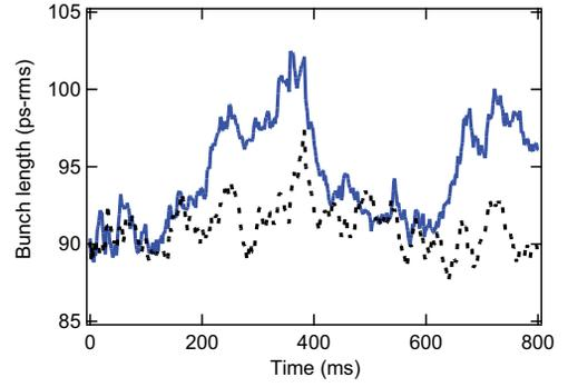
Figure 2: Bunch length measured with the streak camera. Continuous line: a mechanical light chopper at 2 Hz enables periodic laser injection (the laser is seeded during 250 ms at  $f_{rep} = 1$  kHz, and then cut off during the following 250 ms). Dotted line: laser OFF.  $I = 4.8$  mA. The natural bunch length at low current of this measurement is higher than expected because the RF cavity electric field was not optimised. Data are smoothed.
