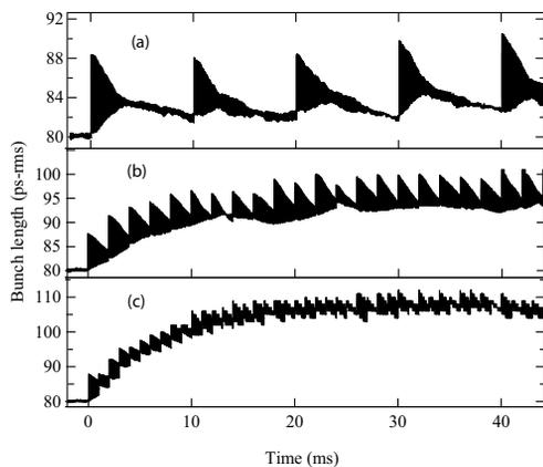
Figure 3: Bunch length evolution from laser OFF to stable CHG operation. (a)  $f_{rep}=100$  Hz,  $T_{90\%} \approx 20$  ms, (b)  $f_{rep}=500$  Hz,  $T_{90\%} = 18$  ms, (c)  $f_{rep}=1$  kHz,  $T_{90\%} = 14$  ms. Simulation with 15000 particles and the parameters of table 1.  $T_{90\%}$  is the time to reach 90% of the bunch length at saturation.
