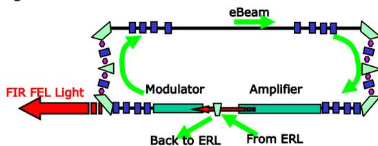
Figure 10: Schematic layout of optics free FEL
