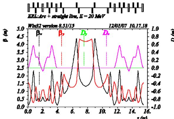
Figure 6: Lattice  $\beta$  and  $D$  functions of the R&D ERL for the case of zero longitudinal dispersion  $D_s = m_{56}$ . The  $m_{12}$  and  $m_{34}$  elements are controlled independently using quadrupoles in the dispersion-free straight section.
