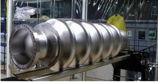
Figure 5: The ERL cavity following BCP at JLab.
